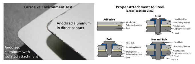
Examples of Metalphoto properly attached to steel with no corrosive degradation.
